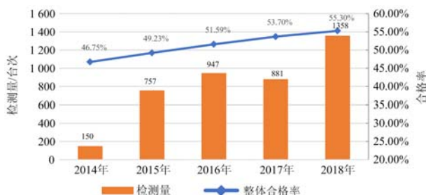
图 4 2014—2018 年充电设施例行检测量与合格率 Fig. 4 2014—2018 qualified rate of in-operation electric vehicle supply equipment
